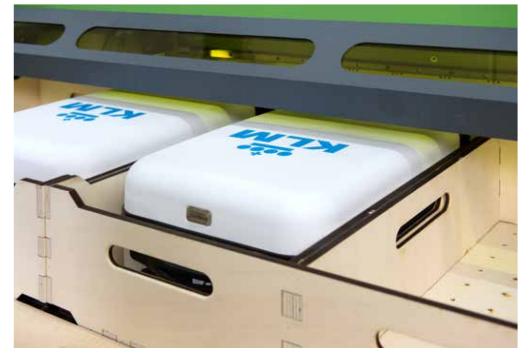
Roland raised its Roland LEJ-640S-F400 UV flatbed printer to accommodate a large construction table underneath to facilitate the printing of multiple cases.
