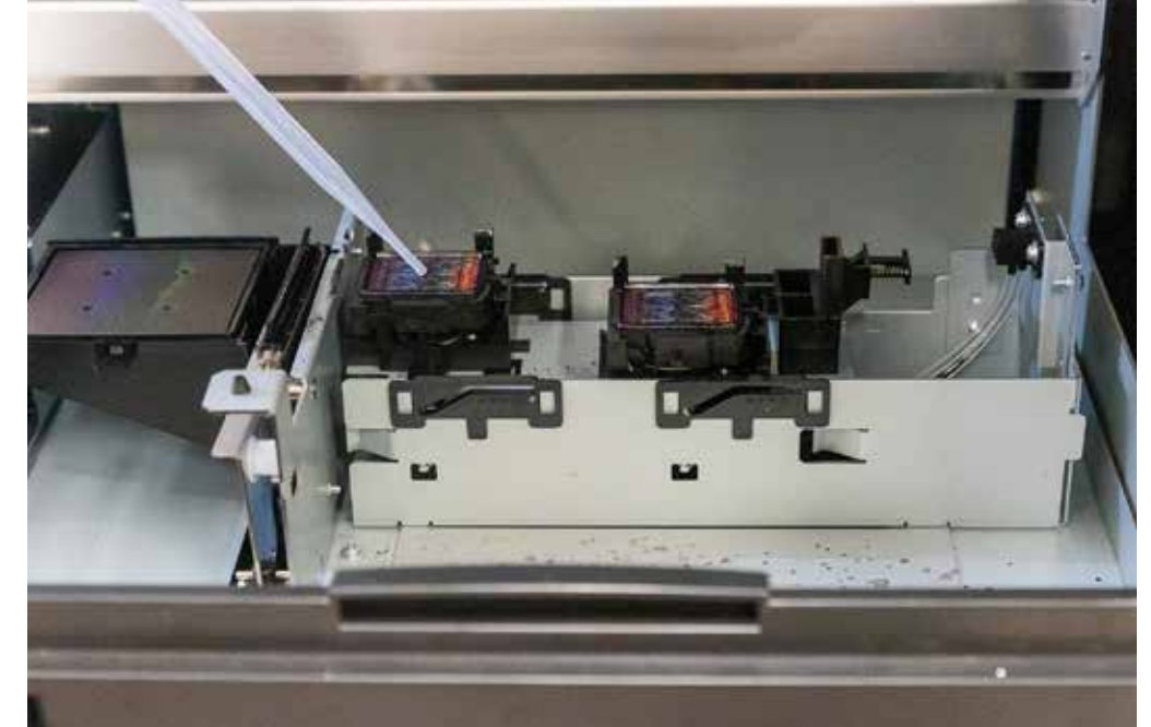
Some of the head maintenance tasks are carried out automatically by the printer. The wipers do need to occasionally be cleaned with cleaning fluid.
