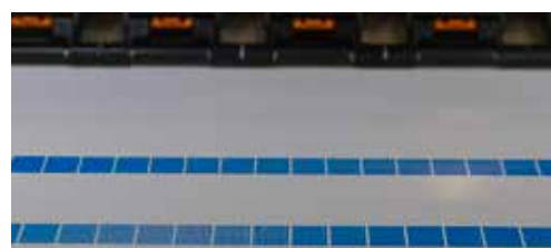
The RGB sensor at the right of the print carriage uses printed patches to adjust the timing in bidirectional printing, if required by the thickness of the material.
