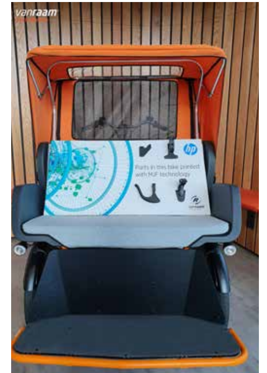
Chat riksja bike Van Raam with 3D printed parts.
