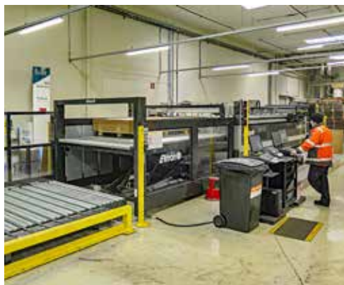
An operator picks up pallets of sheets die-cut with the Elitron Kombo TAV, ready for subsequent bonding, packaging and shipping.
