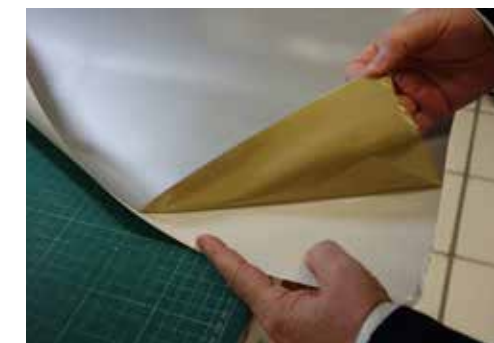
Peel off multilayered cast vinyl on casting sheet.
