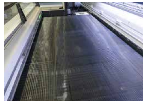
The drying unit can be moved forward to give access to the transport conveyor when the lid is open.
