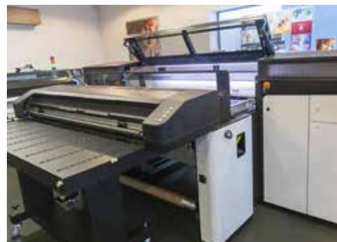
The drying unit can be moved forward to give access to the transport conveyor when the lid is open.
