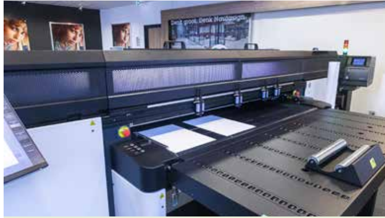
Plates are fed in from the rear. One of the two roll holders for the input of roll material positioned on the table.
