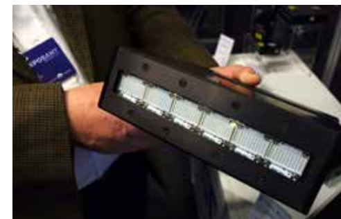
LED UV lamp head made by IST.
