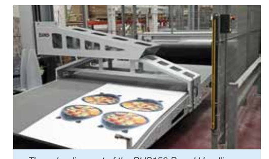
The unloading part of the BHS150 Board Handling System.
