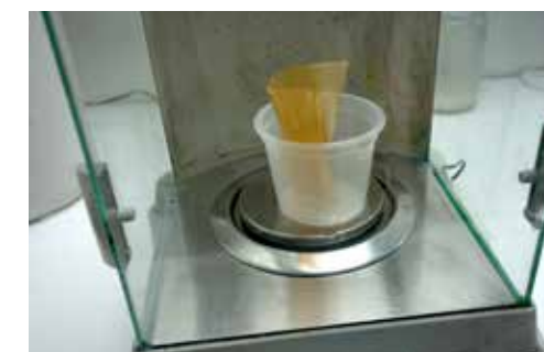
Checking the specific weight of a single cast layer.
