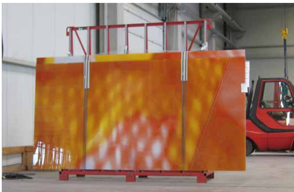
Parts of the design printed with ceramic inks.
