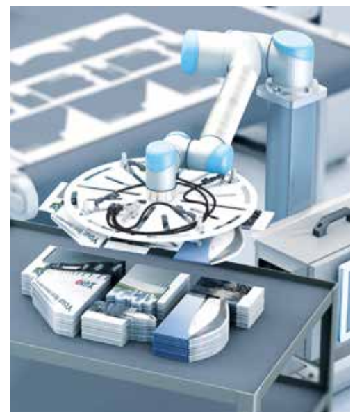
Zünd supplies an integrated, easy to train picking robot, which collects and sorts smaller contour-cut items alongside operators.
